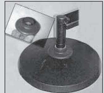
Seal Sealer is an injection-molded plastic cap that's designed to fit over the closing wheel's original bearing seal. "It's easy to install and if the wheel is still good when you spin it, there's no need to replace the bearings," says inventor Rick Heintzman.
