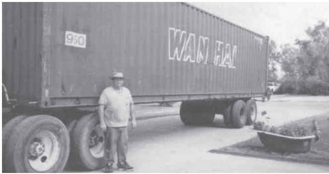
Ray spent about $12,000 turning an 8 by 8 1/2-ft. shipping container into a live floor trailer that he pulls behind his semi tractor. He uses the trailer in his custom hauling business.
