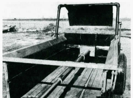
Hydraulically-driven push ram replaces conventional apron and chain to move manure out the tail section.
