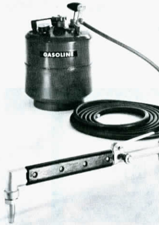
Petrogen torch uses gasoline instead of acetylene or propane.
