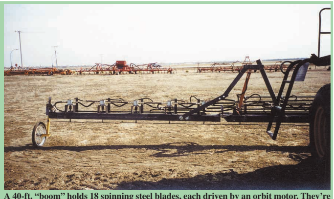
A 40-ft. "boom" holds 18 spinning steel blades, each driven by an orbit motor. They're powered by a separate engine.
