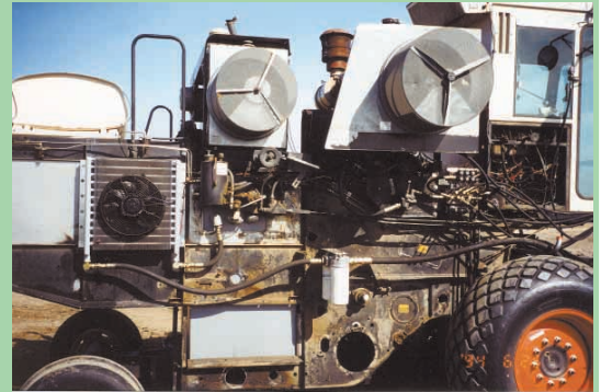
A 40-ft. "boom" holds 18 spinning steel blades, each driven by an orbit motor. They're powered by a separate engine.
