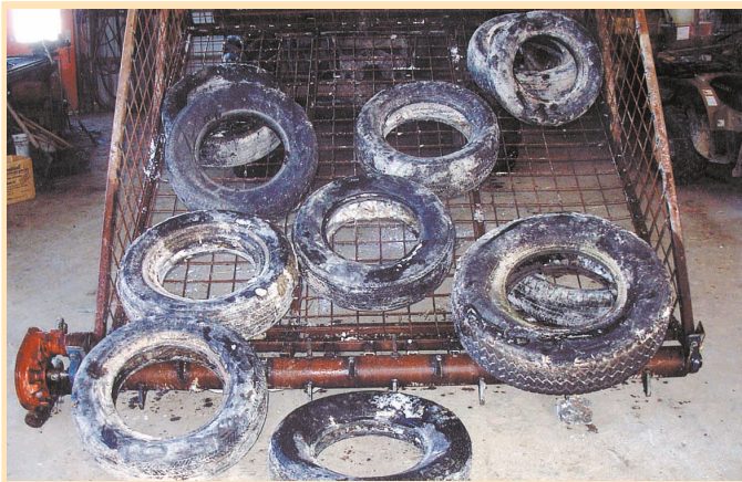
Loader-mounted tire handler, equipped with a rotating shaft on front, pulls tires off the ground and loads them into a metal basket. Shaft is powered by a hydraulic motor.
