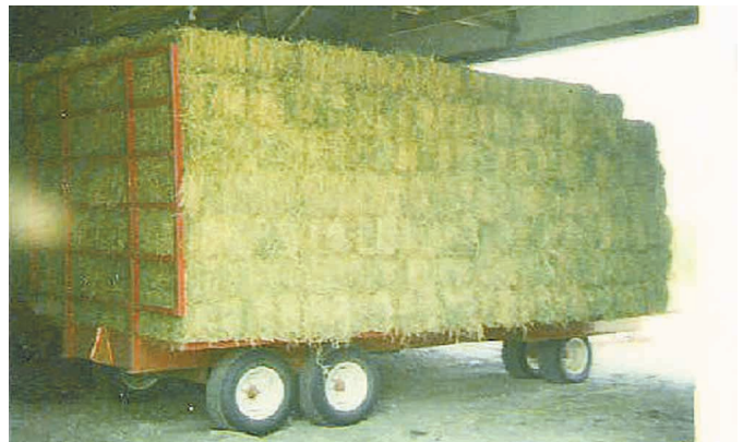
The 9 by 20-ft. wagon has walking tandem axles on back and a dolly wheel assembly on front. The walking tandems allow the wheels to flex instead of the wagon itself.
