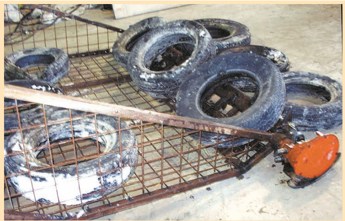
A 2-ft. section on front of basket angles upward to keep tires from catching on beater and kicking back. It also serves as a skid plate.
