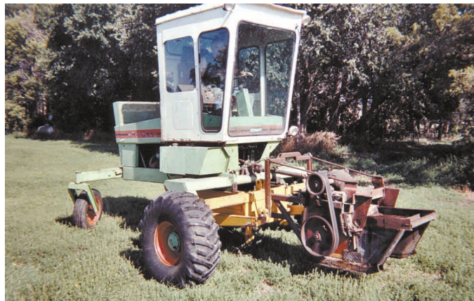
An Owatonna 265 windrower provides the power for Larry Estes's self-propelled tree chopper. It can chew up trees with trunks up to 4 in. in diameter.
