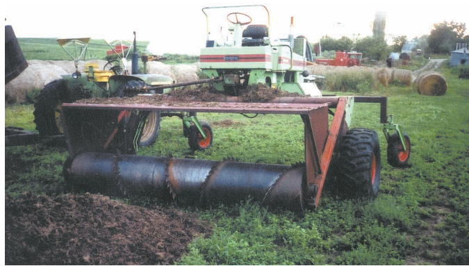
Bill Kleinschmit built this self-propelled compost turner out of an Owatonna 260 swather.
