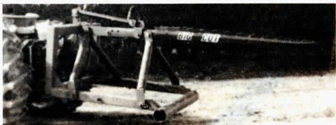
Big bale knife slices upward through top half of bale, putting all the bale's weight on the blade.
