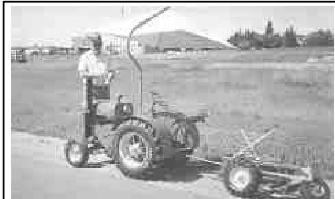
Joel's 1/2-scale 1937 Deere D. The plow depth adjustment levers are made out of bicycle sprockets.
