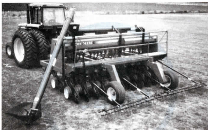
Horizontal 6-in. dia. plastic auger mounts across top of hopper and vertical swing away auger mounts across back of drill.
