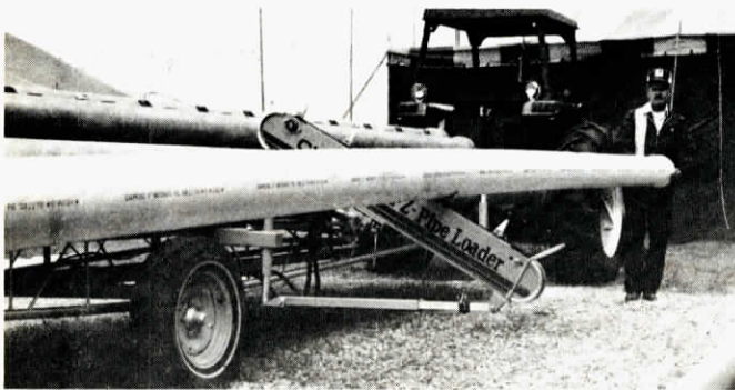
Just roll the pipe on the loader and let the machine's tooth-equipped chain do the rest.
