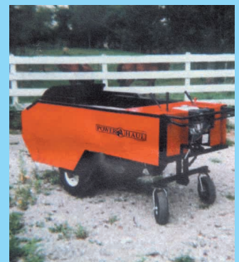
Self-propelled, walk-behind mini manure spreader can haul and spread up to 15 bu. of manure at a time.
