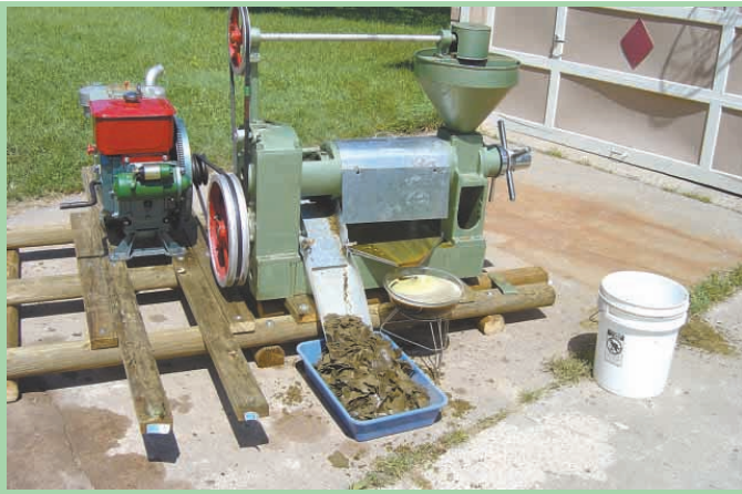
McAmoil uses this Chinese-built screw press to squeeze the oil out of 100 acres of soybeans and sunflowers. A slow speed Listeroid 2-cyl. diesel engine belt-drives the unit.
