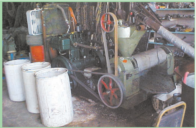
Oil produced by the screw press can be used to operate the Listeroid engine, as well as any other diesel engine on the farm.
