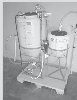
The FuelMeister is a do-it-yourself kit that lets you make up to 40 gal. of biodiesel per day. The closed system eliminates the need to pour or stir liquids.
