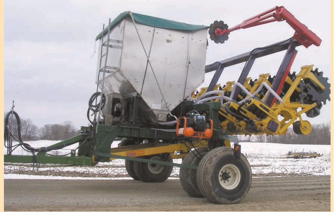
Working with Mark Bauer, Don Bicknese converted his Rawson planter cart into an 8-row Soil Warrior zone tillage machine.
