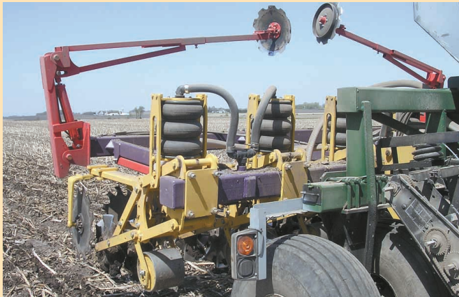
Bauer designed a tilting lift mechanism mounted on 2-in. spindles on back of cart.
