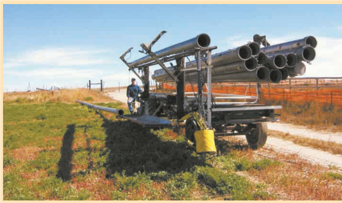
Larry Fulton came up with this self-propelled rig that lets one man lay down and pick up gated irrigation pipe without ever getting out of his seat.
