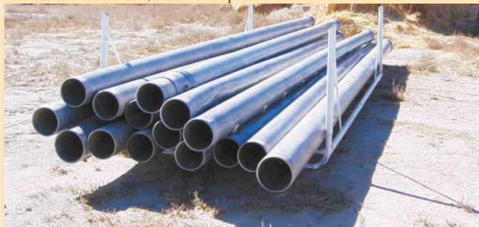
Cradles made from 3-in. dia. pipe are used to hold groups of pipe off the ground. To load the machine, cradle is winched onto machine's self-loading arms.
