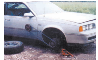
Belt drives a shaft that extends through hole in right front passenger door to another pulley that direct-drives compressor.
