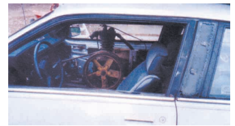
Belt-driven air compressor sits in passenger seat of Rodler's front-wheel drive Oldsmobile car. Compressor is driven by a pulley that mounts in place of car's right front wheel.
