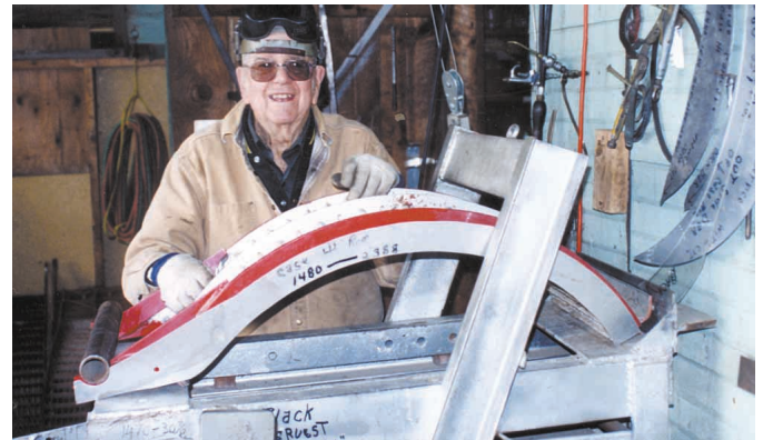
Bill Hickman built a simple hydraulic press to put the curve back into combine concaves. It can be swung in an arc to any spot over the concave, or beneath it.
