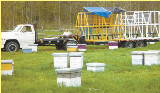
To move a bee cell, Sperlich simply backs trailer under cell and hydraulically raises bed to pick it up off the ground.
