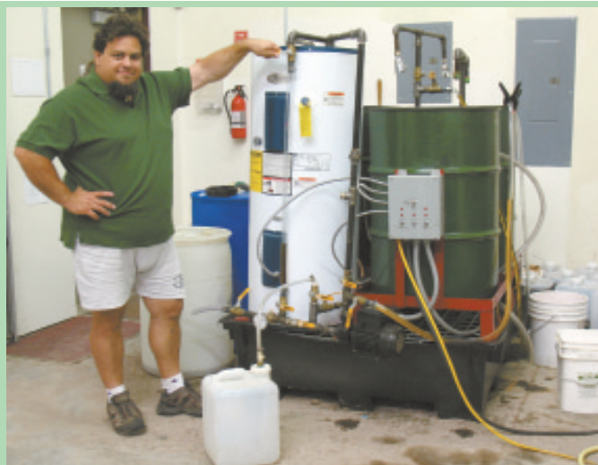
Fugate's biodiesel production system comes with everything you need to start making 80 gal. of fuel in a day. "We've kept it non-automated so it's easy to figure out," he says.
