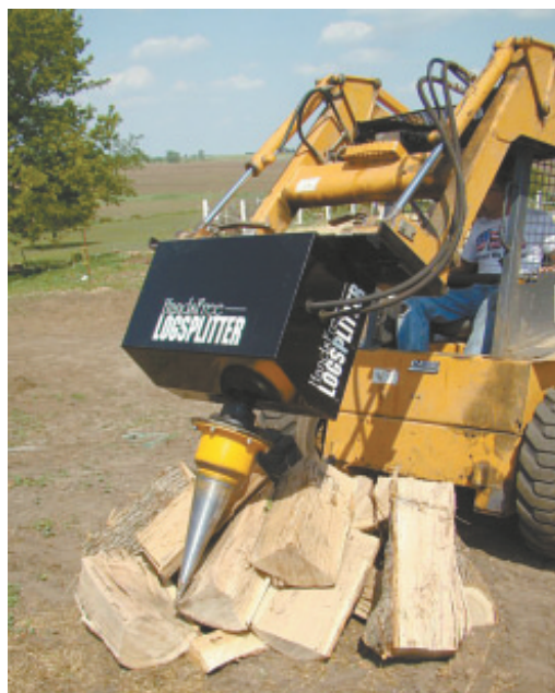
Hydraulic-powered cone-type splitter quick-taches to any skid loader. "It eliminates the need to pick up a log to split it," says inventor Charlie Van Dusartz.
