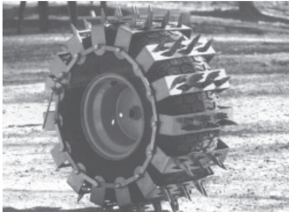
Tim Bowman put nails through rubber belting to make his first Mow-Aerator.
