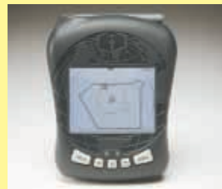
System includes a handheld receiver unit and a weatherproof GPS transmitter unit that attaches to dog's collar.
