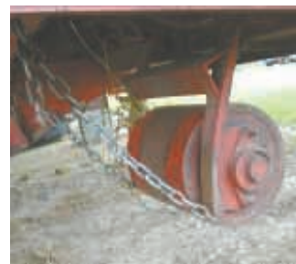
Ruhlen stalk rollers knock stubble over before it can tear up tires. Chains keep the roller from going back under the header if the combine backs up when header is down.
