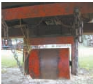
Ruhlen stalk rollers knock stubble over before it can tear up tires. Chains keep the roller from going back under the header if the combine backs up when header is down.
