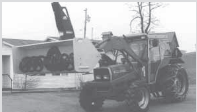
Doug Webster converted his pto-driven Erskine snowblower to hydraulic power, eliminating an underslung driveshaft that led from tractor's rear pto to the up-front blower.
