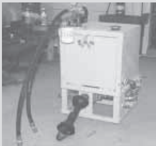
Blower is driven by a 30 gpm hydraulic motor that attaches to back side of blower. The motor is driven by hydraulics from a pto-driven pump (shown in photo) that mounts on back of tractor.
