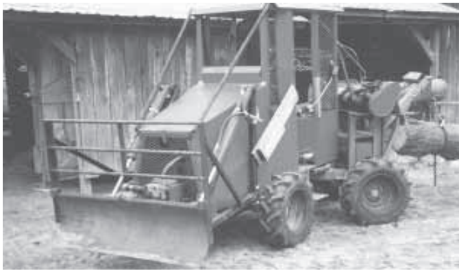
Lloyd Lohman's home-built 4-WD log skidder is completely hydraulic and articulates in the center.
