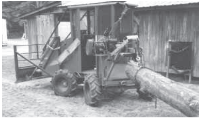
Winch is made from a 1932 Chevrolet car transmission. It drives a 3/8-in. dia. cable with hook.
