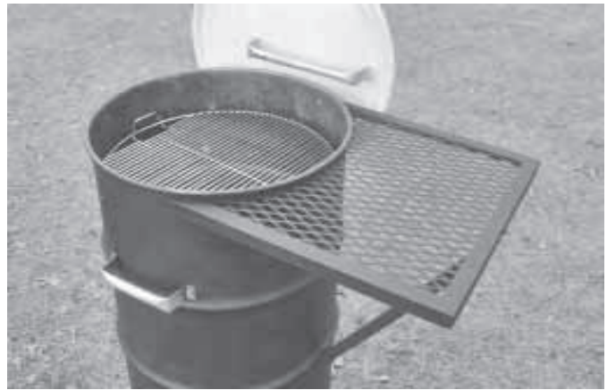
"Grill-n-Barrel" is made from a used 55-gal. steel drum.
