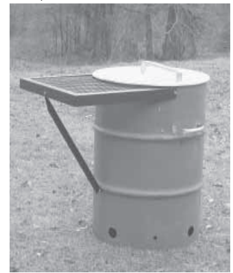
Vent holes at bottom of drum and a metal lid on top are used to control the draft.
