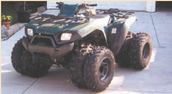
Mark Bader added duals all the way around on his 2005 Kawasaki 650 4-WD ATV. He bought four new "deep mudder" tires and rims and mounted them on the inside, moving the original wheels to the outside. Each set of wheels is separated by pvc spacers and held in place by four long bolts.
