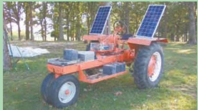
Tractor is powered by a 15 hp electric motor, with two banks of batteries recharged by a 50-watt solar panel.
