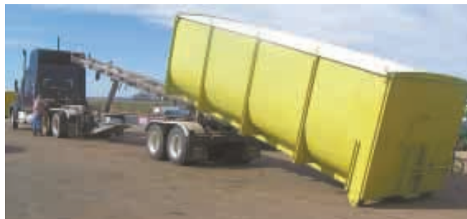
Tarp-protected hoppers are transported by a special-built trailer.
