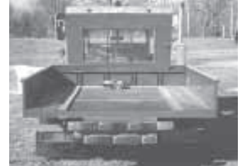
The rig has dual wheels on back. The bed is raised and lowered by a 12-volt hydraulic pump that acts on a 3-in. dia. cylinder with a 16-in. stroke.
