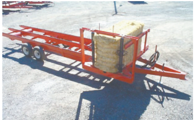
Flake feeder will feed large size square bales up to 2,000 lbs.
