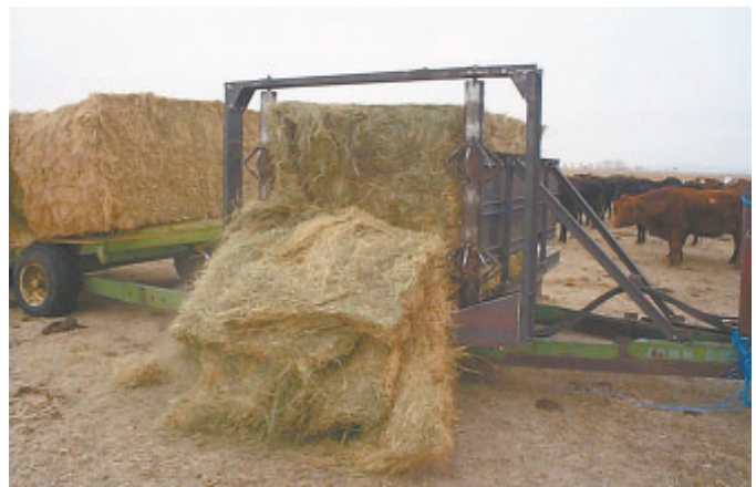
Fodder-Flake Feeder lets one person feed hay without getting out of the tractor cab, except to remove bale strings. Large rotors peel off sections of hay.
