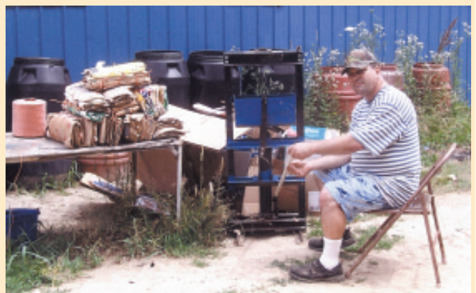
Phil Orlovski modified a small hydraulic press to convert cardboard - and other household paper waste - into fuel for his wood stoves.
