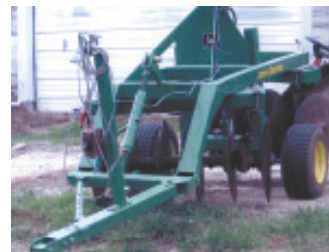
Matt Richter built a mini scraper and a tandem disk for about $200 each. Both implements are equipped with electric actuators and are sized to be pulled by an ATV or garden tractor.
