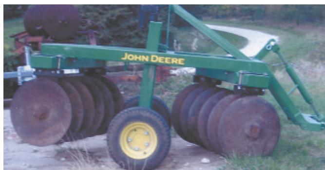
Matt Richter built a mini scraper and a tandem disk for about $200 each. Both implements are equipped with electric actuators and are sized to be pulled by an ATV or garden tractor.
