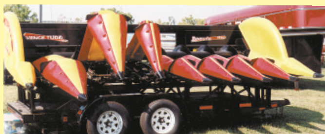
Row width on new corn header is adjusted by changing the inserts on snouts (in yellow) and sliding gathering chain units back and forth.
