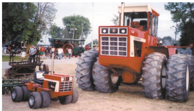
"I built this 1/4-scale, 4-WD, articulated tractor to look just like my dad's 1976 IH 4366 model," says Todd Rufenacht.
