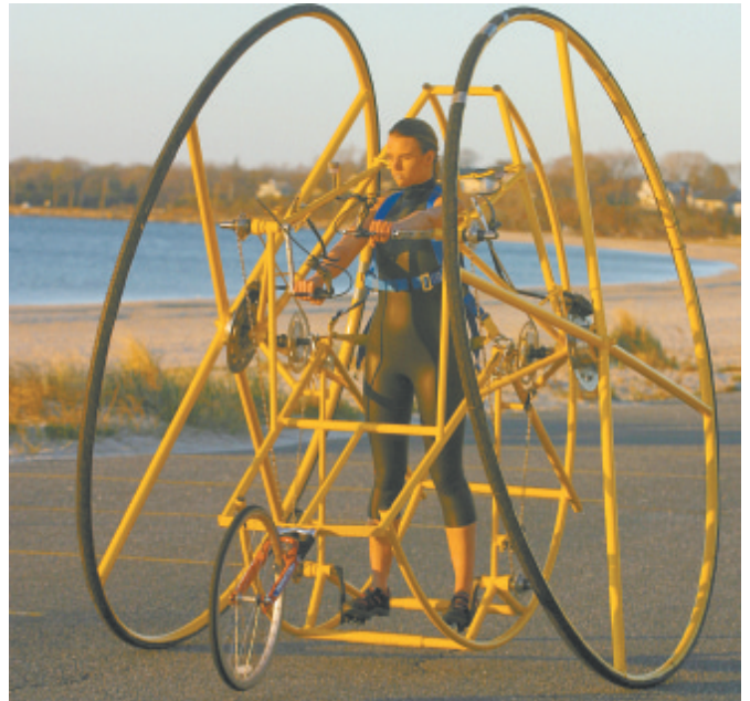
With no seat, the HyperBike gives the user “a full body workout,” as it requires use of both arm and foot pedals. The driver uses a “skate-ski” motion to propel it.
