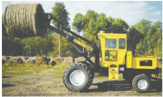
John Fehr uses salvaged combine components and used Chevy engines to build his special “Fehr-Trac Loader” tractors.
