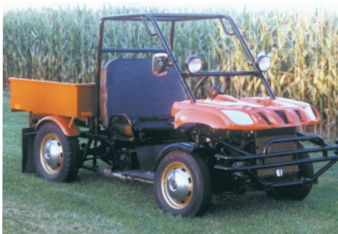
"I had a lot of fun building it, and my family and I enjoy riding it around our farm," says Stanley Smiley about the utility vehicle he built out of a 1964 Fiat 2-WD car.
