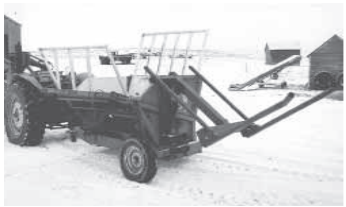
Rear forks load bales into shredder, eliminating the need for a second loader tractor.
