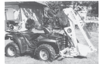
Bill Ganswich designed this backhoe for his 1994 Suzuki 250 ATV. The boom swings 60 degrees and can dig 6 ft. deep.
