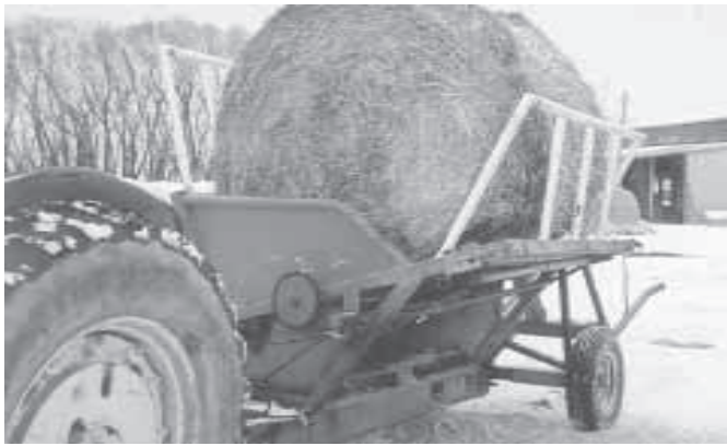
Lewis Hacault started with a sprayer cart and ended up with this home-built bale shredder.
