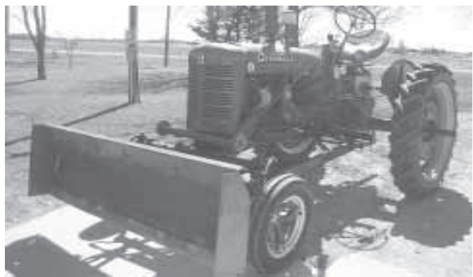
Home-built 7-ft. blade mounts on front of Ken Anderson’s IH Super C tractor.
