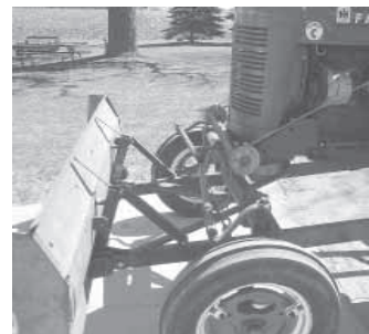
A pair of lift cables run over pulleys on front of tractor.
