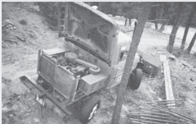
Overhead photo shows side-by-side engines and crab steering, which helps maneuver around obstacles.
