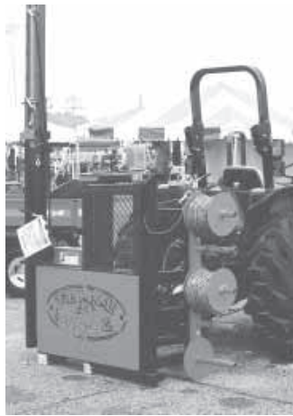
Fence Dawg fencing equipment is available in four different models. All are hydraulic-operated and equipped with a unique braking system. T-post driver mounts on the side (at left in photo).
