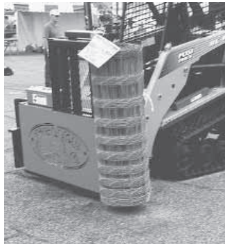
Skid loader-mounted model can unroll and stretch up to three standard barbed wire rolls at a time or one roll of woven wire fence.
