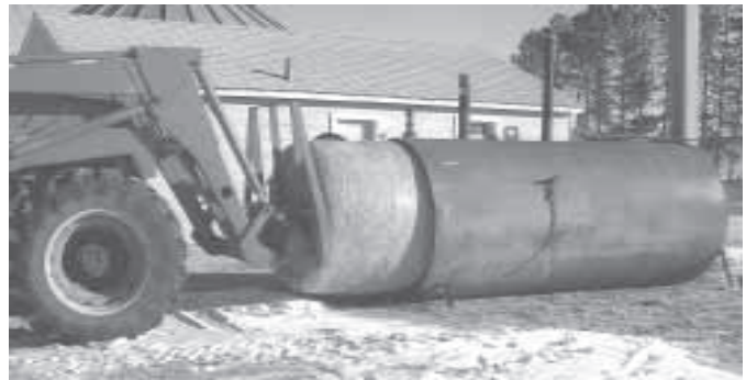
Residue burner was built from a 1,000-gal. underground fuel storage tank.
