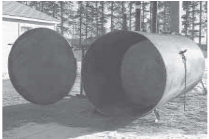
He used angle iron and a piece of 1/2-in. pipe to make hinges so he could cut off one end to serve as a door.
