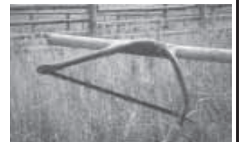
Duct tape fastens 20-in. bow saw to a length of pvc pipe.
