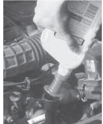
Oil Buddy has a spring-loaded valve that opens and closes the spout.
