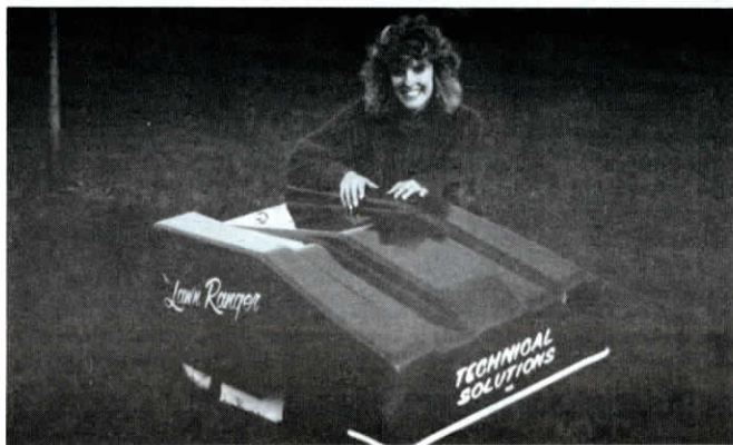
Self-guided "Lawn Ranger" shuts itself off if anything touches the outside casing.
