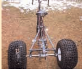
Two separate chains are used to drive bike's limited slip rear axle.
