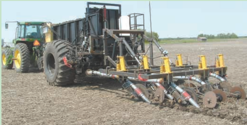
First-of-its-kind machine compresses manure and drops it into deep trenches via flexible 3 1/2-in. dia. augers.
