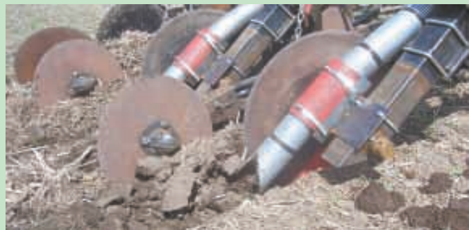
Trench is opened by 24-in. dia. coulters. A trailing 18-in. disc closes it up.
