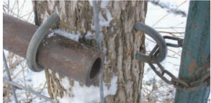
Giant staples are made out of 1/2-in. dia. steel rod salvaged from old silo hoops.
