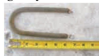
Staple is made from a 14-in. length of rod bent into a U-shape.
