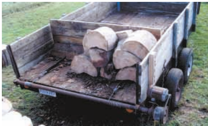
Wood panel that pushes wood chunks off back of trailer is powered by a winch and cables that wrap around pipe at back of wagon.
