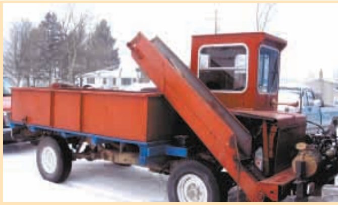
Built on the frame of a Chevrolet Blazer, the machine is equipped with a hydraulic-operated splitter on front and a 10-ft. long conveyor on one side that drops wood into a wagon box.
