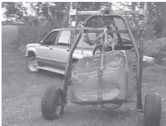
Only about 6 in. of the rock in this photo was originally above ground. Edes used a shovel to dig the rock out, then used the log hauler to lift it up and away.
