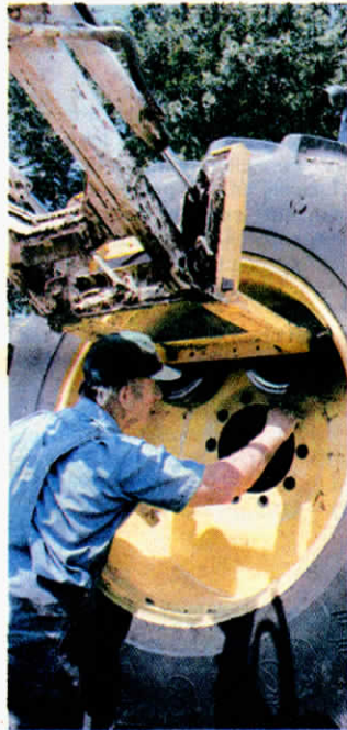
Tractor dual, riding on attachment's small wheels, is easily spun by hand to align bolt holes.
