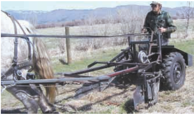
In-line mower can be pulled by horse or subcompact tractor. "Works great for getting rid of weeds between trees without using chemicals," says inventor Marvin Brisk.
