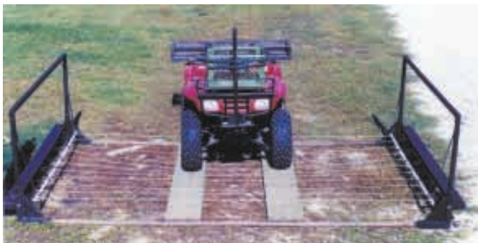
“Hot” cattle guard is tied into an electric fence and floats a few inches above the ground.
