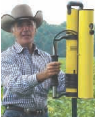
Dennis Tippmann says his propane-powered fencepost driver is powerful enough to slam T-posts into frozen ground.
