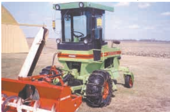
Anderson added brackets to snowblower arms to match the arms on the swather.
