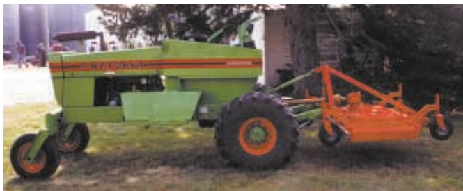
“Thanks to its hydrostatic drive, it works great for mowing and blowing snow,” says Charlie Anderson, who converted an Owatonna swather into a mower/snowblower.
