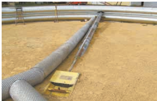
Kevin Holst's auger system is designed to clear corn out of his 18,000-bu. pile, which is contained inside a 60-ft. dia. temporary storage bin.
