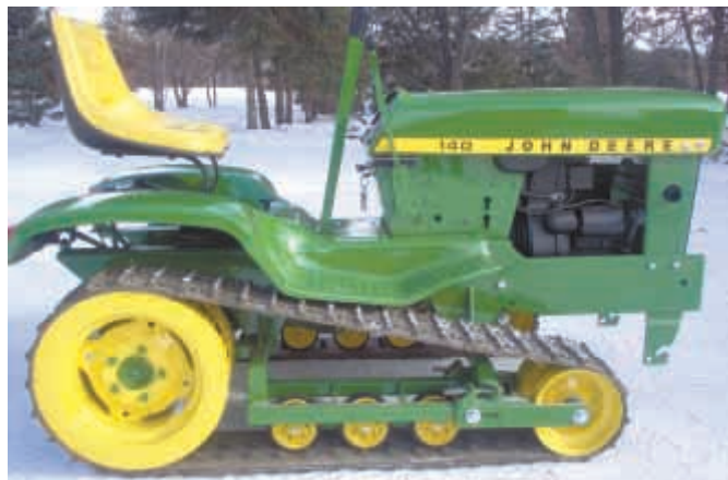
Todd Poach added tracks to his Deere garden tractor by slicing a track from a Deere snowmobile in half lengthwise and building a custom track system.
