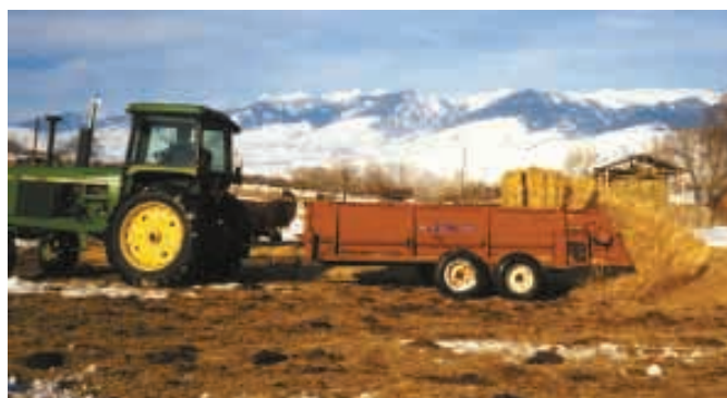
Ordinary manure spreaders can be used to spread big square bales out onto fields or in livestock pens.
