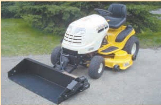
Johnny Bucket is a self-contained lifting system that allows owners of smaller riding mowers and garden tractors to add a loader.
