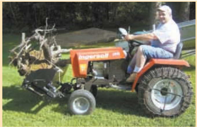
Battery-powered "power dump" empties bucket. A manual dump is also available.
