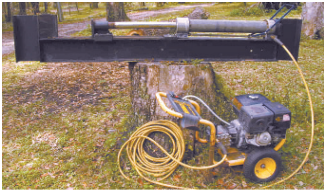
Paul Behm uses a pressure washer to power his new log splitter.
