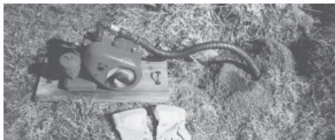
Portable gopher gasser makes use of an old motor. Flexible metal tubing runs from motor's exhaust into tunnel.
