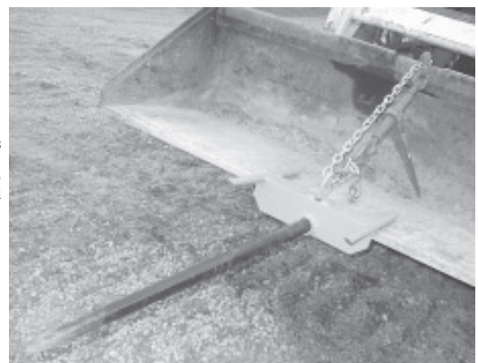
Bracket slips over cutting edge of bucket to securely hold bale spear.
