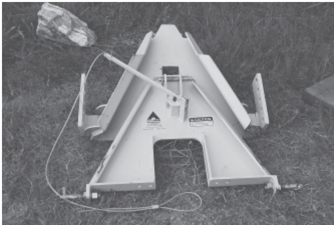
Control plate mounts on tractor's 3-pt. hitch and slides into a receiver plate that attaches to implement.
