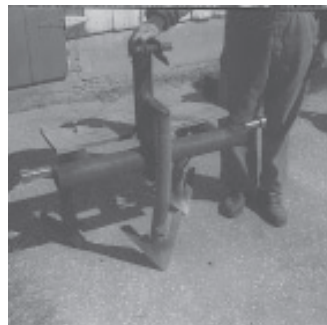
Miller's 3-pt. mounted chisel plow is just 3 ft. wide and is equipped with three sweeps off an old row crop cultivator.
