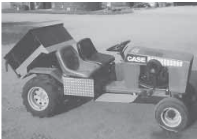
Marion Schultz stretched out his Case 446 tractor, adding a passenger seat and a hydraulic-operated dump box on back.
