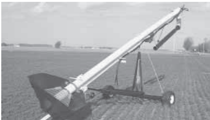
Sliding auger support makes it possible to span 45 ft. without repositioning auger.
