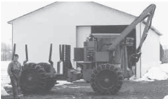
Log-loading tractor has a front-mounted boom that swings to either side.
