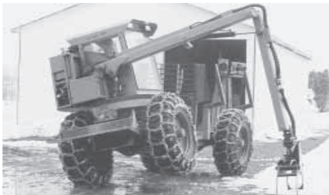
Cab and boom rotates 180 degrees, allowing operator to load logs on back.
