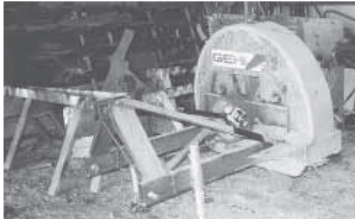
Pitcher made this 3-pt. mounted rotary ditcher by cutting the bottom out of an old Gehl silage blower. He used 2 by 6 box steel to make a 3-pt. mounting bracket.
