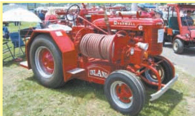
Super A “Fire Tractor” was built in 1956 by IH, but outfitted for firefighting by another firm. Added gear included a 150-gal. water tank and a reel with 200 ft. of hose.
