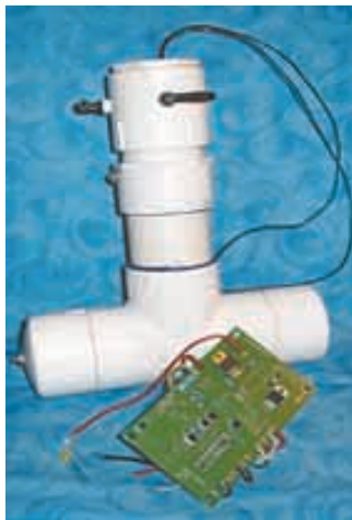
Kit feeds a mix of hydrogen and oxygen into air filter.
