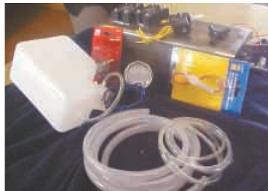
Photo shows all components needed for new mileage booster. Water reservoir, left, feeds water automatically to hydrogen-generating unit, right.
