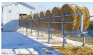
A line of straw bales are fed continuously into heating system on a conveyor.
