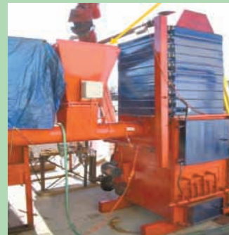
Bales are chopped and carried into furnace by conveyor.
