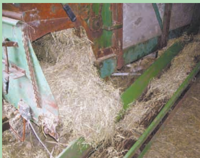
Bales are chopped and carried into furnace by conveyor.
