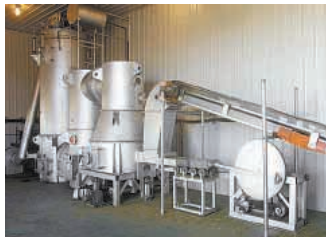
Vidir biomass greenhouse heating system can be used anywhere hot water can be pumped.
